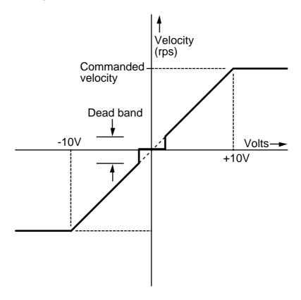
Figure 3-13. Analogue Differential Input Characteristic
